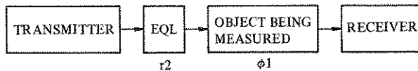
Figure ① AM-PM Conversion Coefficient Measurement According to Standard Group-Delay Network Method
